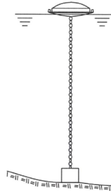
The thickness of its chain shall be 8mm and it should be vertical and stretched. When rope is used, it should be of equivalent durability (breakage limit = 13.9 kN or 1.42 tons) and it must be vertical and stretched. The minimum required weight, in order to not shift is 20 kilograms. There could be used two pavement plates, the weight of each is 12.5 kilograms and total weight of  $2 \times 12.5 = 25$  kilograms. In this way, the weight requirements are overlapped.
